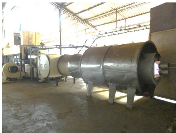
(a) Tea dryer coupled with burner
