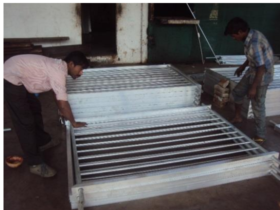
(a) Frames and collector pipes
