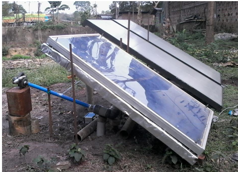
Fig. 15 TU SHAG II (1.2m ×1.8m) and IITB SHAG (1.2m ×2.4m) test set up at Chandraprabha Tea Factory, Golaghat
