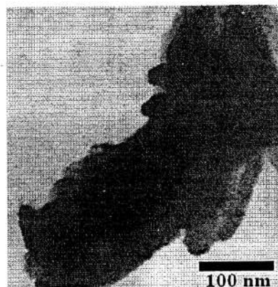
Figure 3: Agglomeration of the nanorods at the highest fluence
