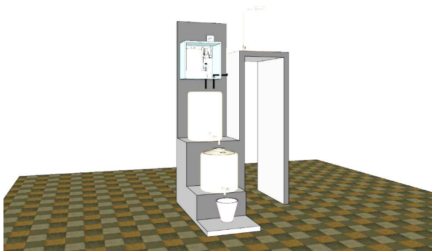
Fig.5.vii.a: Schematic diagram of the dosing unit for Fluoride Nilogon
