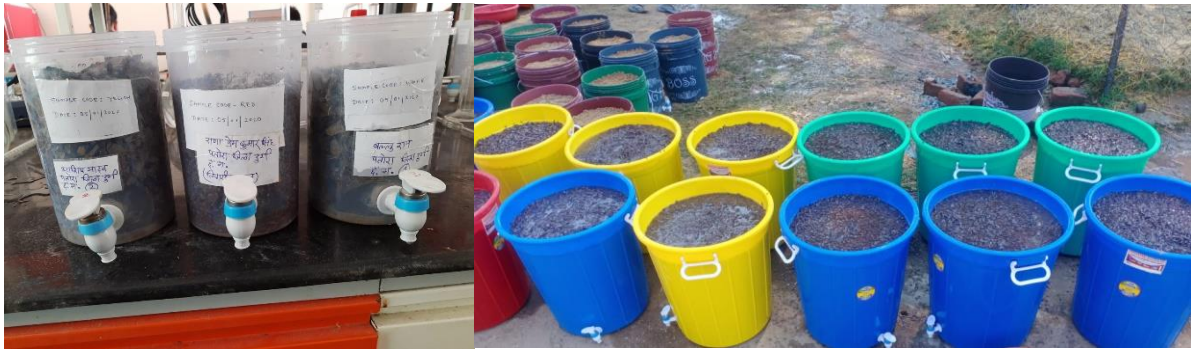
Fig.2.iii.b2. Limestone from Durg being tested at PI's laboratory in TU (left) and Reactors of some of the 100 household Fluoride Nilogon filters of second phase being installed in Kanker.
