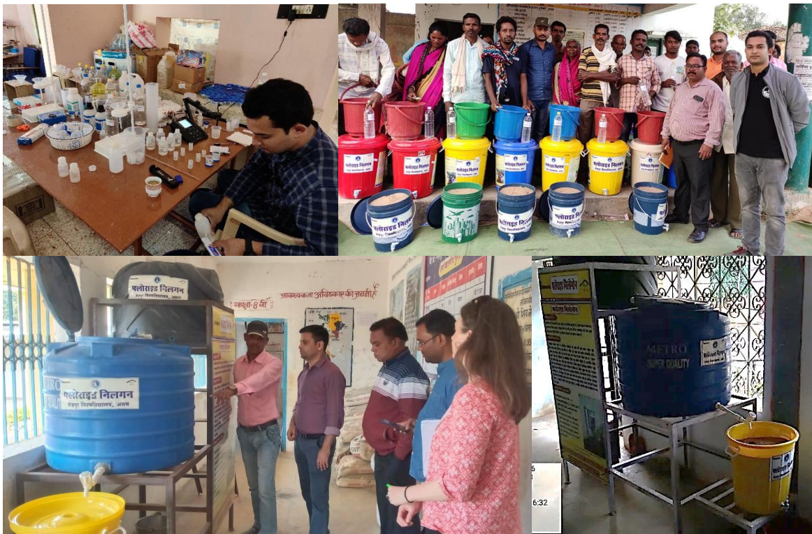
Fig.2.iii.b1. A temporary laboratory with one of the project staff (top left), some of the 19 (15 L) household Fluoride Nilogon filters ready for distribution to villagers in front of Dumarpani Panchayat office (top right) and two 88 L small community Fluoride Nilogon filters installed at M.S. Dumarpani Middle School (bottom left) and Dumali Middle School, Dumali (bottom right) in Kanker district of Chhattisgarh.
