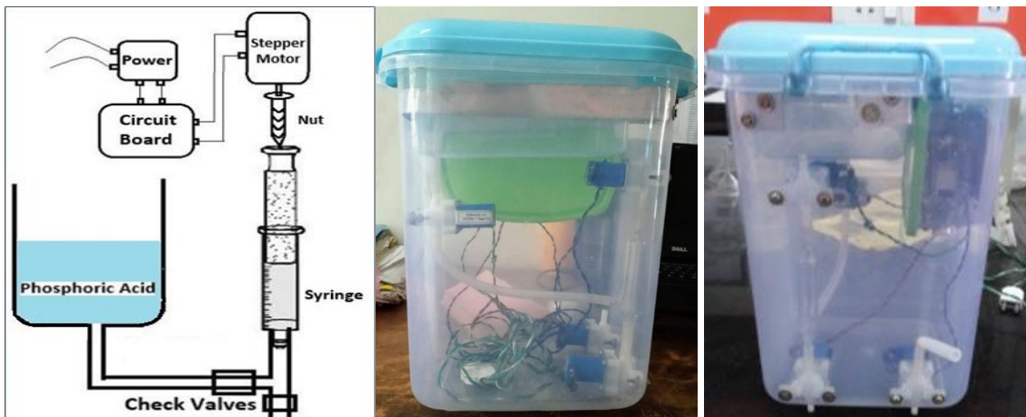
Fig. 2.ii. Schematic diagram, front and rear views of the dosing unit for fluoride Nilogon.
