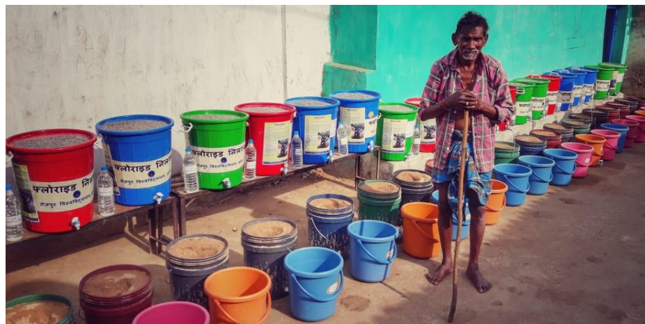
Fig. 2.iii.c. Some of household Fluoride Nilogon filters installed at Khariyar and Dhuruapada villages near Khaira in Nuapada district of Odisha.
