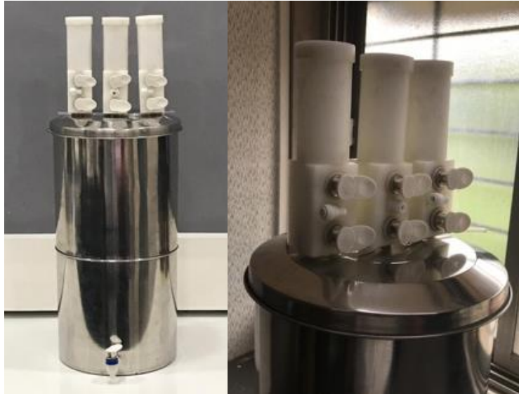
Fig.2.i. Prototype of Arsiiron Nilogon filter designed with Prabha Technotrade, Bombay
