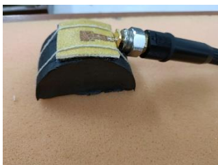
Figure 4: MPA testing on the developed phantom
