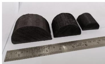
Figure 3: Hand phantom developed using graphite powder (Make - Merck) mixed with silicone rubber (Make - Moldsil) in the weight ratio 1:1.
